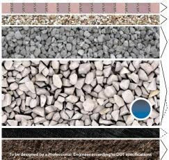
Borgert Pavers 31/s" (80 mm) Thick Permeable Joint Material (ASTM NO. 8, 89 or 9 Aggregate) Open-graded Bedding Course 11/2 to 2" (40 to 50mm) Thick ASTM NO. 8 Aggregate (3/8 inch)
