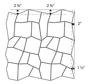
Note: There are 6 layers per cube at 12.68 SF per layer. Layer dimension is  $44\frac{3}{4}$ " x  $41\frac{3}{4}$ ".
